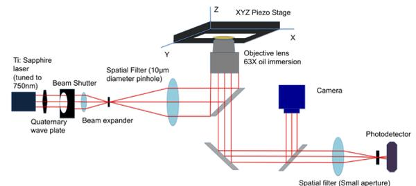
**Figure 1.** Two-photon lithography system layout: This layout shows the path of the beam as it travels from the laser, through the microscope to expose a sample, and into the camera and photodetector.
