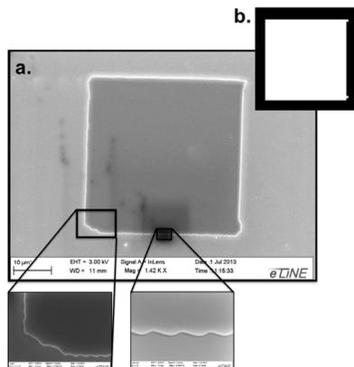
**Figure 2.** Fabricated square structure: (a) SEM image of the fabricated square structure. (b) Resized binary image template used to create the different structures in 2a.
