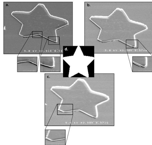
**Figure 3.** Fabricated Star Structure: (a) Tilted SEM image of the first star structure. (b) Tilted SEM image of the second star structure. (c) Tilted SEM image of the third star structure. (d) Resized binary image template that was used to create the star structure in 3a-3c.
