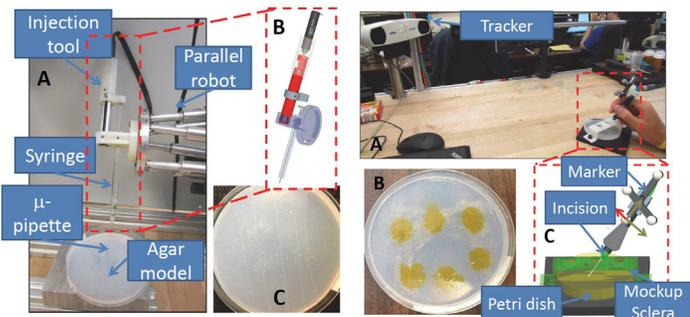
**Figure 1.** Panels ABC (left) demonstrates the vessel cannulation while panels ABC (right) shows the membrane peeling process.
